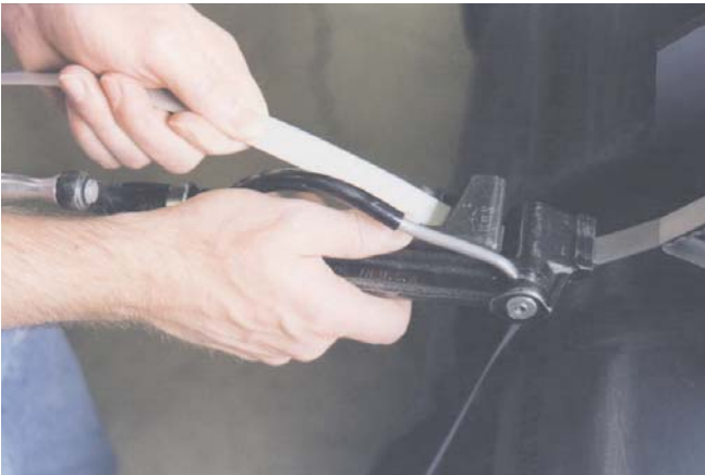
17. Holding the tool slide against the tool nose, pull the strapping back until the tool nose presses against the seal.
