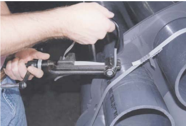
21. Open the cutting handle. This action will trim the excess strapping.
