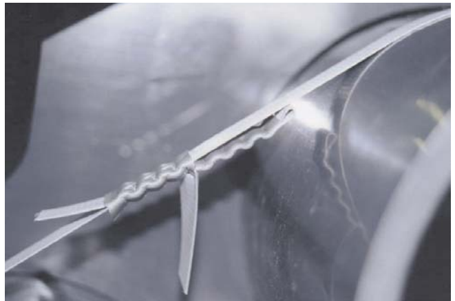
22. Above is a close-up view of the sealed strapping joint.
