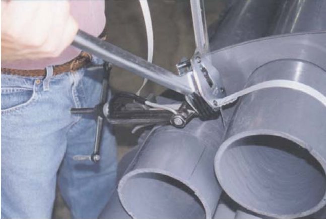
19. Place the open sealing tool over the seal.
